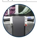
Acceleration of forward/backward movement is proportional and positioned near the basket raising and lowering button, to enable these movements even during forward movement. All systems are operable without having to move the hand from the accelerator, for maximum operator comfort.
