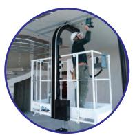
Activated directly from the platform with a push of a button, the sheet travels up the track into the overhead position, then retaining the drywall sheet in the proper location, leaving the worker free to screw or nail it to the joists/studs.
